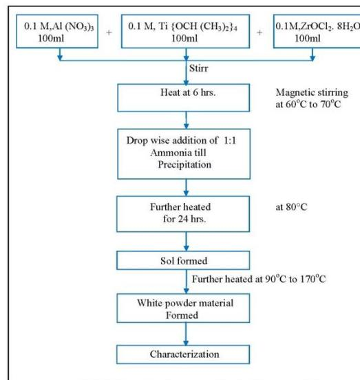
Fig. 3.2 Flow sheet diagram of  $\text{AlTiZrO}_4$  nanomaterial
