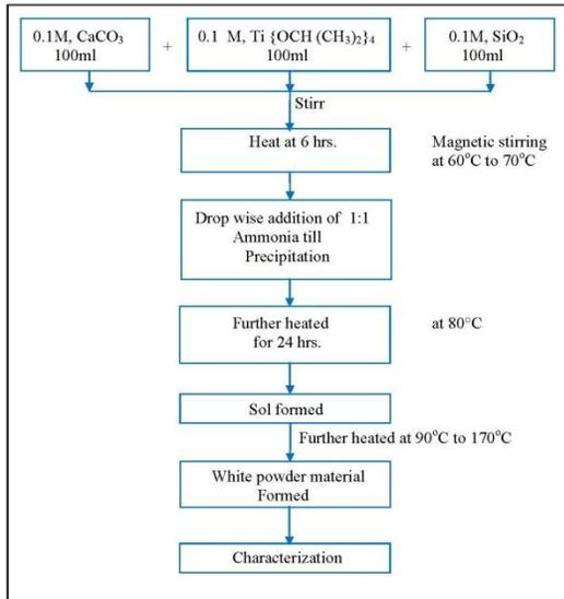
Fig.3.1 Flow sheet diagram of  $\text{CaTiSiO}_5$  nanomaterial
